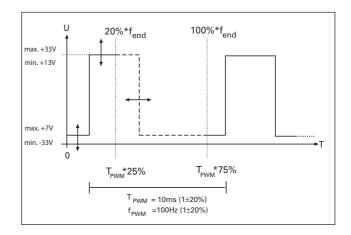
If no signal is present the pump runs up to its final rotation speed.
