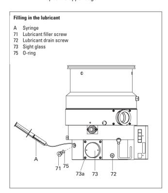
⇒ Screw back in lubricant filler screw 71 with the 0-ring 75.
