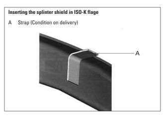
→ Before insert the splinter shield in the CF-F flange the strap must be bent.
